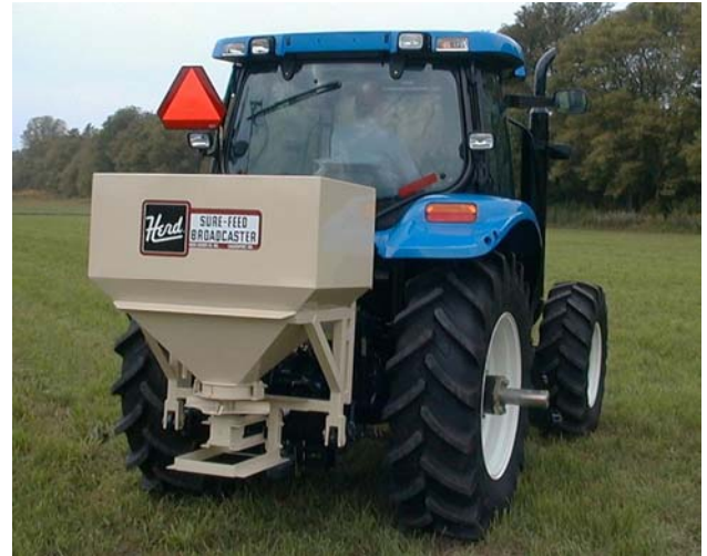
Model 1200C 3-pt. For Category 2 Tractors 1200 lbs. capacity-20 cubic ft. – 16 bushels
