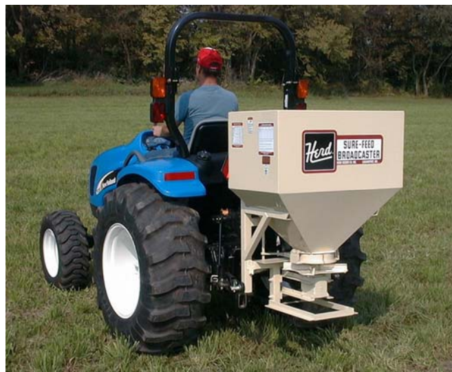
MODEL 750 3-PT. FOR CATEGORY 1 TRACTORS 750 lb. Capacity-9.6 bushels-12 cubic ft.
