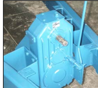
2-speed gearbox for better mixing power
