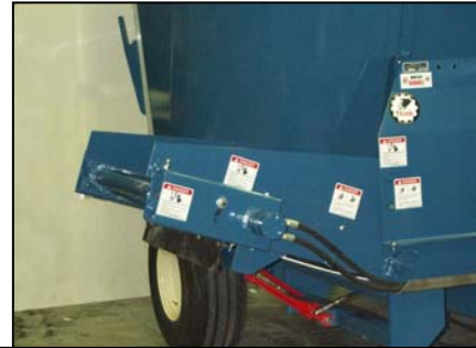
Hydraulic raise and lower discharge conveyor extensions
