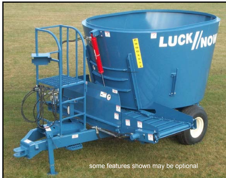
standard side discharge with slide chute
