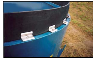
9" rubber extension for larger capacity mixes
