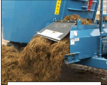
Hydraulic cross conveyor to feed both sides
