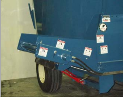
Hydraulic raise and lower discharge conveyor extensions
