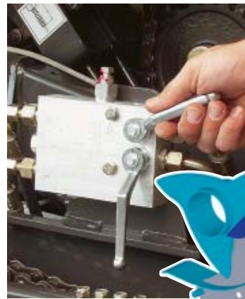
HydroProtect knife protection
