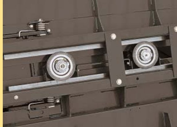
Large diameter externally mounted plunger drive rollers
