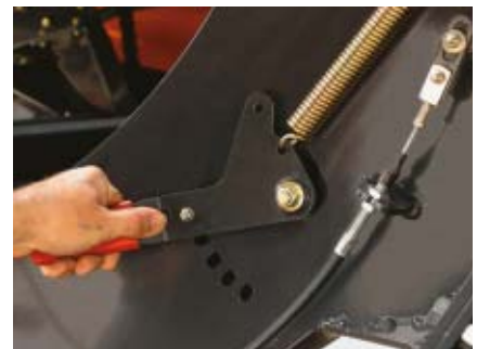
The pre-chamber pressure can be finetuned according to different conditions
