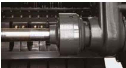
Torque limiter on packer drive
